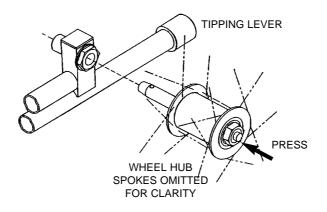
Ensure the brake is not applied. With one hand hold the frame of the wheelchair and with the other hand hold the spokes surrounding the hub and fully depress the centre button pulling the wheel away from the wheelchair axle bush and releasing the centre button.
